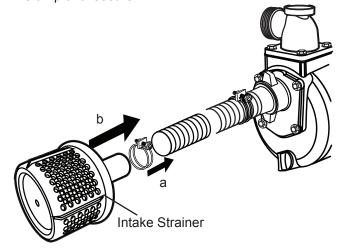
5. For the discharge hose, slide a Hose Coupling Ring over the remaining Hose Coupler (a) and place a Gasket onto the end of the Hose Coupler (b).
